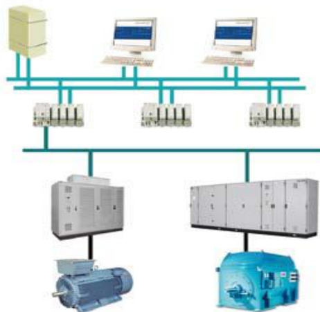
Fig.4. Connecting motors with local network-connected converters.
