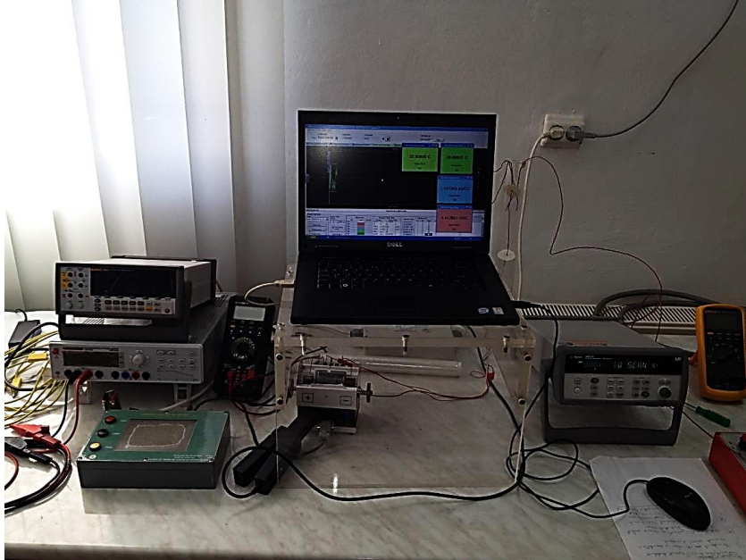
Fig. 3. Test rig for maximum surface temperature of the cells
